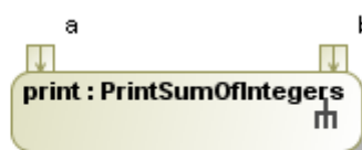
Figure 53 -- Creating a Print Action by Dragging the PrintSumOfIntegers Opaque Behavior to Activity Diagram
